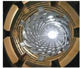
Inoex's vacuum calibration tank uses lattice-like interwoven steel straps to change pipe length and diameter over a 4:1 range.
