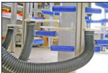
Make cleaner food and medical films with Kdesign's patented air-exhaust system, which prevents oily condensation on the bubble cage.
