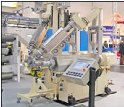
Davis-Standard's new coex cosmetic-tube line uses Knoedler's compact four-motor CMG drives on each of four extruders.
